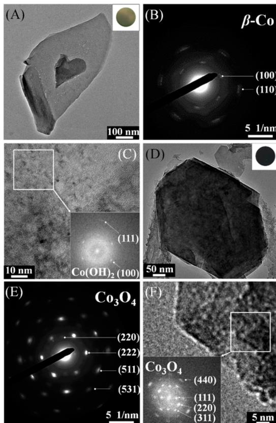
**Figure 3.** Morphology and SAED pattern images. (A) TEM image, (B) SAED pattern, and (C) HRTEM image of  $\text{CoO}_x$ . (D) TEM image, (E) SAED pattern, and (F) HRTEM image of  $\text{CoO}_x$  after the OER scan (after two times of LSV in the range of 1.0 to 1.7 V). Insets: (A, DE) color of their corresponding catalyst surfaces; (C, F) FFT image of their corresponding regions.
