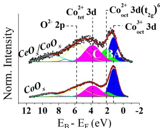
**Figure 8.** Valence bands for  $\text{CoO}_x$  and  $\text{CeO}_x/\text{CoO}_x$  at 1.4 V. The Co fitting results are labeled as A (blue), B (green), and C (pink), respectively, for the calculation of relative area ratios. The data were collected using a photon energy of 130 eV for the valence band. A Shirley background was subtracted from the spectrum before deconvolution.
