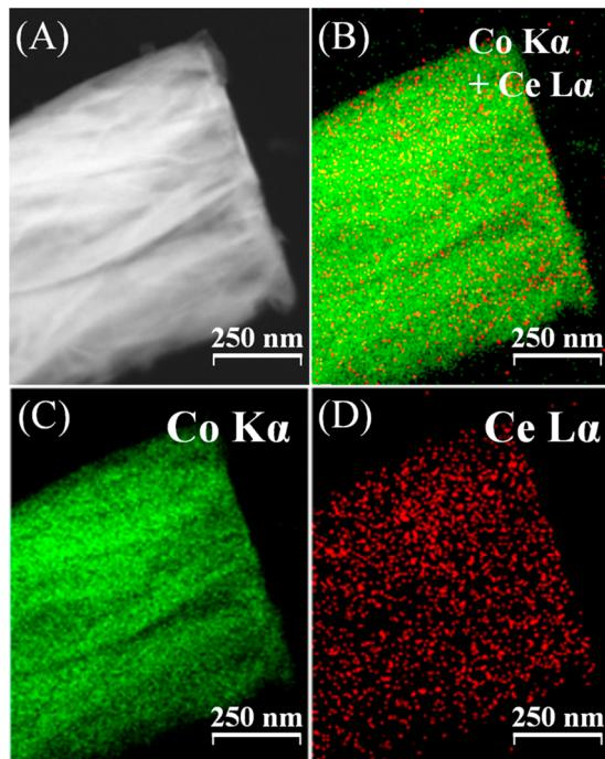
**Figure 4.** (A) STEM image and (B–D) the corresponding EDS elemental mapping of the  $\text{CeO}_x/\text{CoO}_x$ . The TEM specimen was prepared by sonicating a film-type catalyst with ethanol for 10 min.
