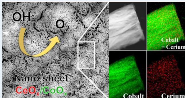
the electronic structure of surface Co species (facile formation to  $\text{CoOOH}$ ) on the  $\text{CoO}_x$  catalyst and optimizes the binding energy of intermediate oxygenated adsorbates.
