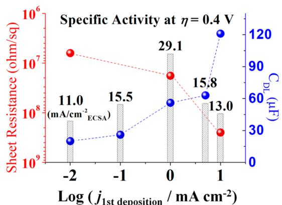
**Figure 1.** Correlation of the specific activity with the sheet resistance and electrochemical double-layer capacitance ( $C_{DL}$ ) of the various first steps of Co deposition conditions for the Co-based catalyst.
