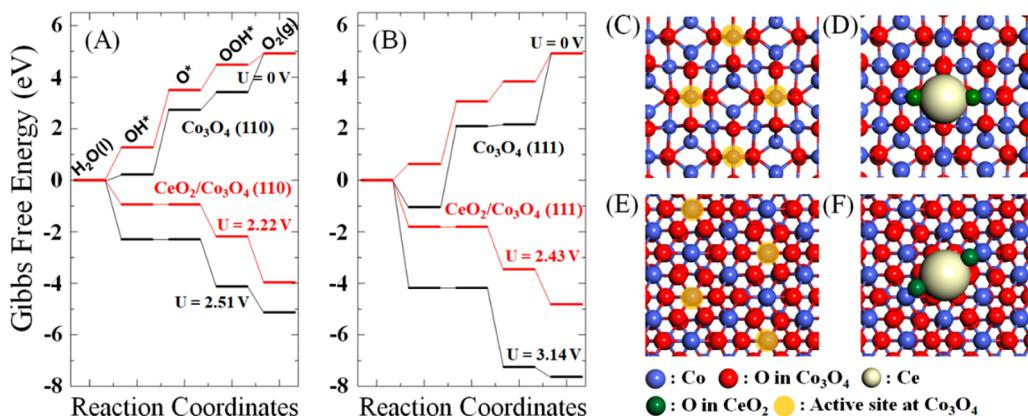
**Figure 9.** Gibbs free energy diagram for OER with the  $\text{Co}_3\text{O}_4$  and  $\text{CeO}_2/\text{Co}_3\text{O}_4$  systems with (A) (110) and (B) (111) surfaces. Slab models with the active site highlighted in orange: (C)  $\text{Co}_3\text{O}_4$  (110), (D)  $\text{CeO}_2/\text{Co}_3\text{O}_4$  (110), (E)  $\text{Co}_3\text{O}_4$  (111), and (F)  $\text{CeO}_2/\text{Co}_3\text{O}_4$  (111).
