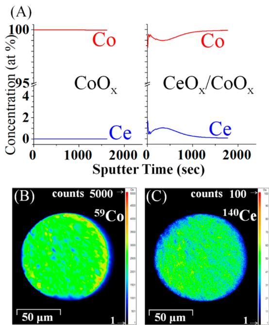
**Figure 5.** (A) SIMS depth profiling of CoO<sub>x</sub> and CeO<sub>x</sub>/CoO<sub>x</sub> 2D images at the surface of the elemental distribution of (B) cobalt and (C) cerium in the CeO<sub>x</sub>/CoO<sub>x</sub> catalyst.
