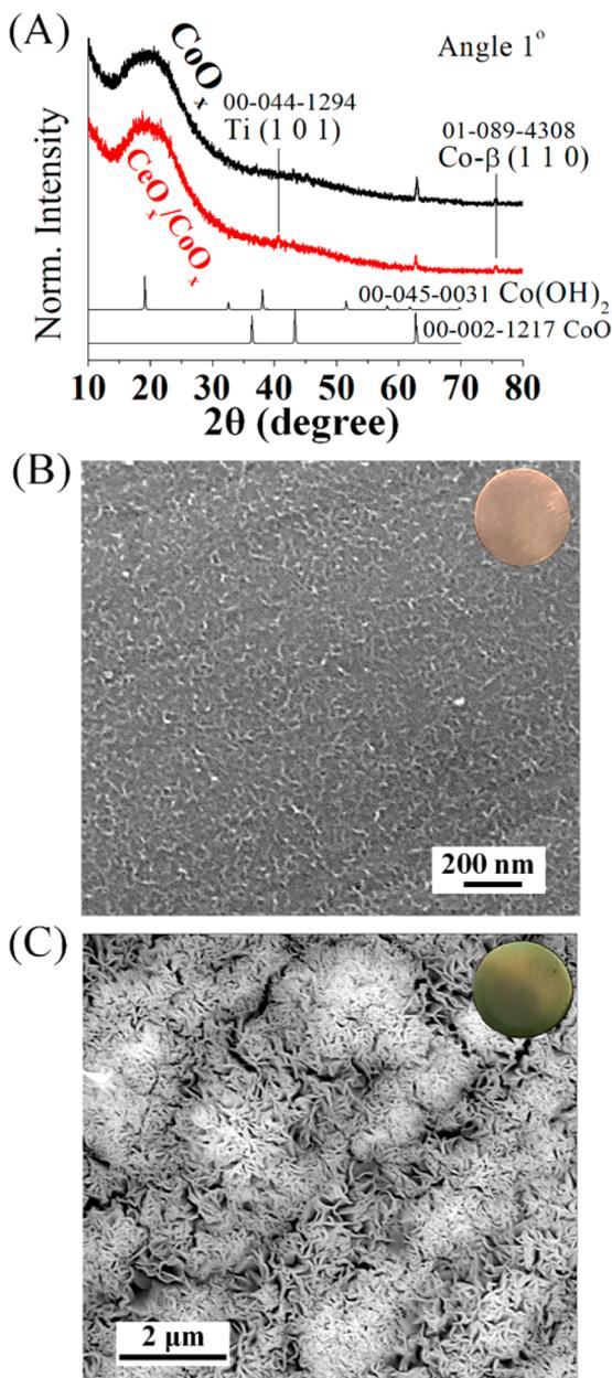
**Figure 2.** (A) Glancing angle X-ray diffraction pattern of the  $\text{CoO}_x$  and  $\text{CeO}_x/\text{CoO}_x$  catalysts. SEM images of surface morphology of (B) after the first-step of Co deposition (Co seed) and (C) the  $\text{CoO}_x$  catalyst (after second-step of Co deposition). Insets in (B, C): catalyst color images.
