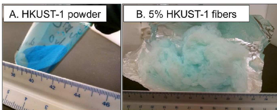
Fig. 3. Images of (A) as-synthesized HKUST-1 powder and (B) HKUST-1 embedded polystyrene fibers.
