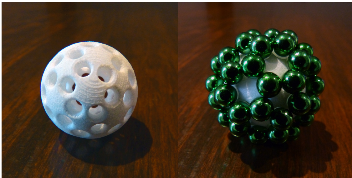
Figure 8: A 3D printed scaffold, and a buckyball of buckyballs arranged upon it.
