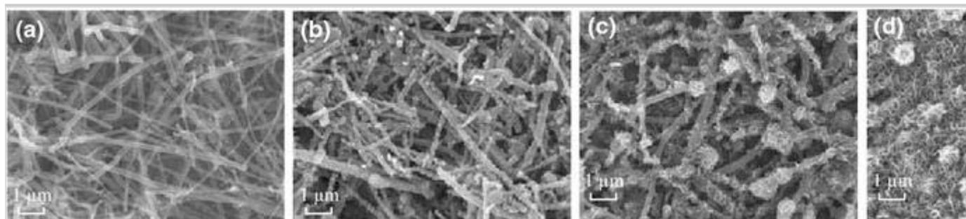
For 5 min growth period (Fig. 1b), only sparse EOG flakes were observed, which do not provide enough surface area. However, when the growth time was increased to 10 min (Fig. 1d), highly dense EOG flakes were deposited, blocking the macropores that are necessary to facilitate rapid ion transport for high-frequency response. The perpendicular orientations of 3D EOG flakes that encircle each CNF can be clearly observed with graphene edges exposed. We selected a growth time of
