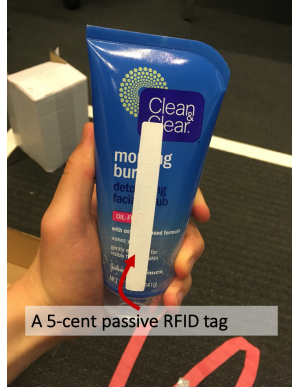
Figure 2—An RFID-tagged object. We attach a battery-less RFID sticker to an object in order to localize it.
