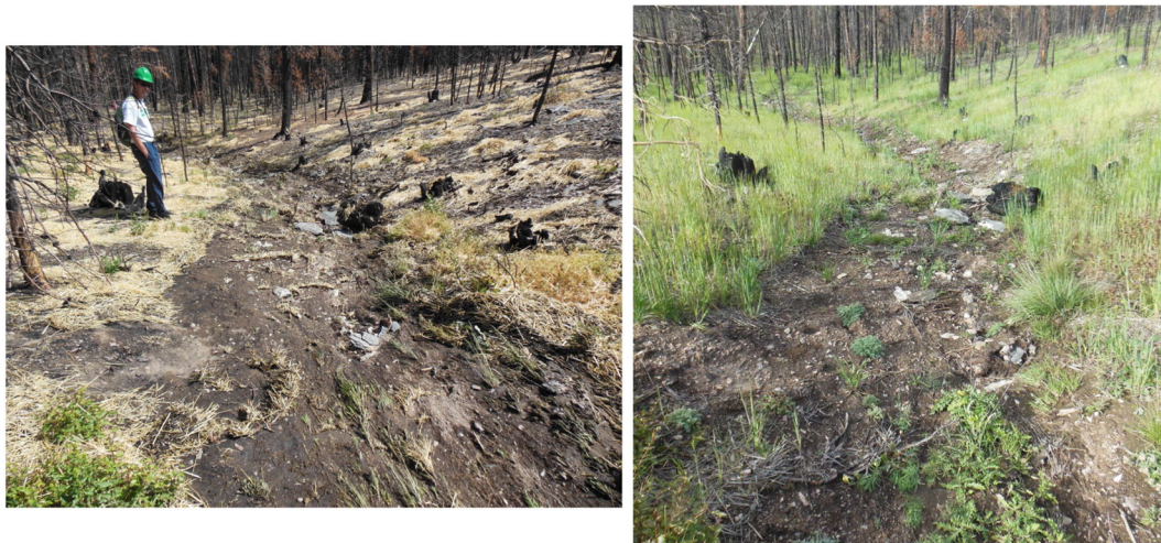
Fig. 10. Repeat photos of an ephemeral channel showing mulch effectiveness where it was retained after a storm on 1 Jul 2013 in the fully mulched watershed of the South Fork Cache la Poudre basin (left photo) and on 17 Sep 13 (right photo). View is downstream.
