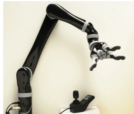
Fig. 4. The Kinova JACO 3 Finger robot.
