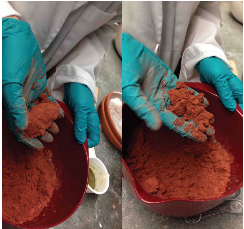
9 The Making and Knowing Laboratory, the ‘squeeze test’ for moulding with sand in a frame, following Ms. Fr. 640, f. 118v. Photos: Emogene Cataldo and Julianna van Visco. [Moulding sand contains previously used ground moulds (made from plaster and ground brick) held together with egg-white binder (f. 82r).]
