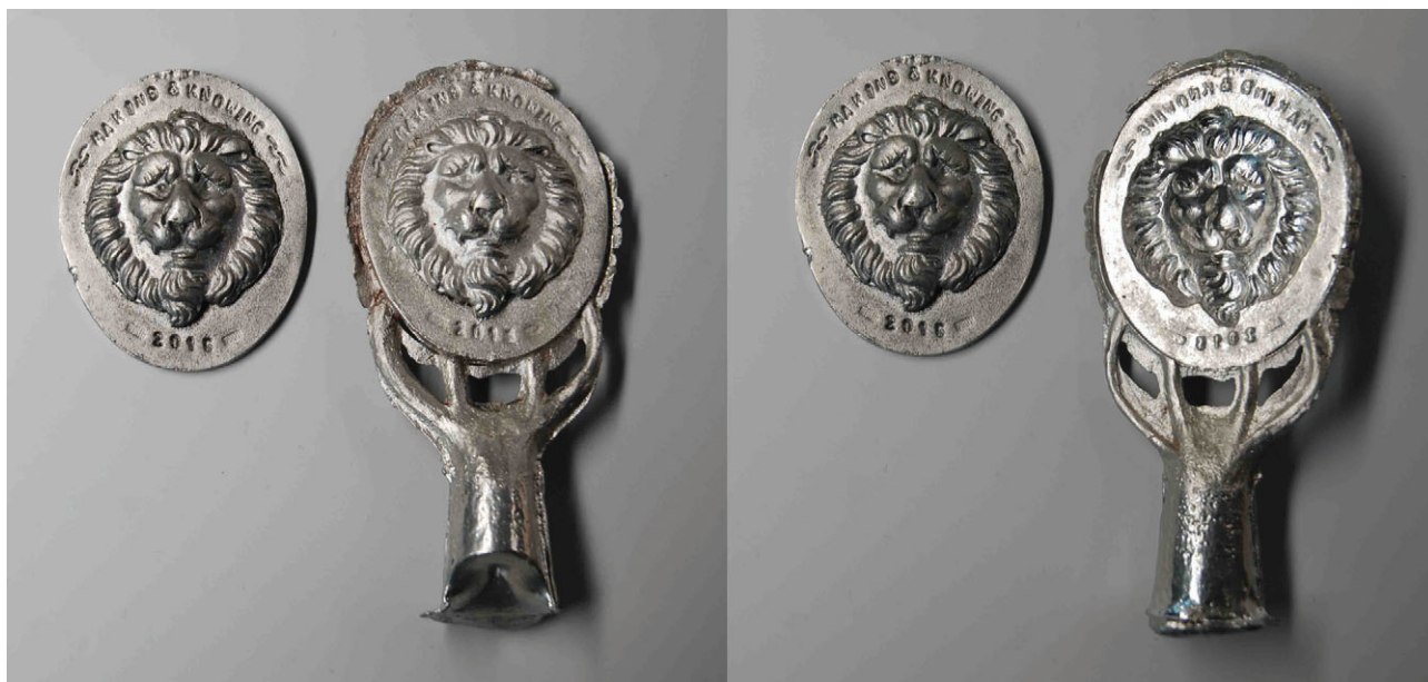
6 Medal pattern and convex side of medal (with casting infrastructure still attached) [left]; and pattern and concave side of medal [right]; following Ms. Fr. 640, f. 92r ('Moulding a hollow on one side and on the other a relief' [known today as 'incuse reverse casting'], the result of experiments by Michaela Groeneveld and Marianne Nuij, University of Amsterdam. Photos: Tamar Davidowitz, The Making and Knowing Project, University of Amsterdam.
