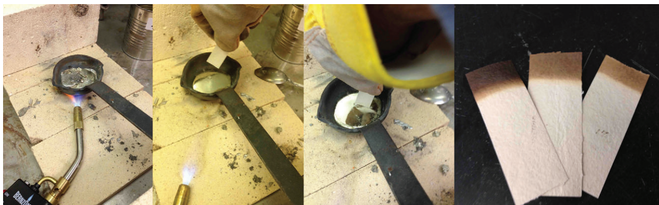
8 The Making and Knowing Laboratory, the paper test. Photos: The Making and Knowing Team, Columbia University. ['To know when it (the 50–50 tin–lead alloy) is the right temperature (for casting into cuttlefish bone), dip a little piece of paper in it. If it turns black without catching fire, it is the right temperature. But if it burns and makes a fire, it is too hot'. The paper employed in this experiment is made from 50–50 hemp and cotton, heavy weight, gelatin sized, and of third quality, used in the repair and conservation of rare books, and supplied by Timothy Barrett, University of Iowa Center for the Book.]
