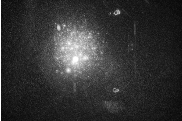
Figure 1. Photograph of an End Test Mass; Exposure time of 1.3 seconds. Light blobs are interpreted as surface dirt. The rings and faint straight lines on the right side of the image are part of the mirror support structure.
