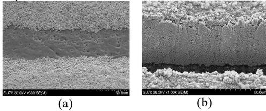
Figure 1. Tilted top view of slot on CB028 layer. (a) Micro-dispensed slot. (b) Laser machined slot [6].
