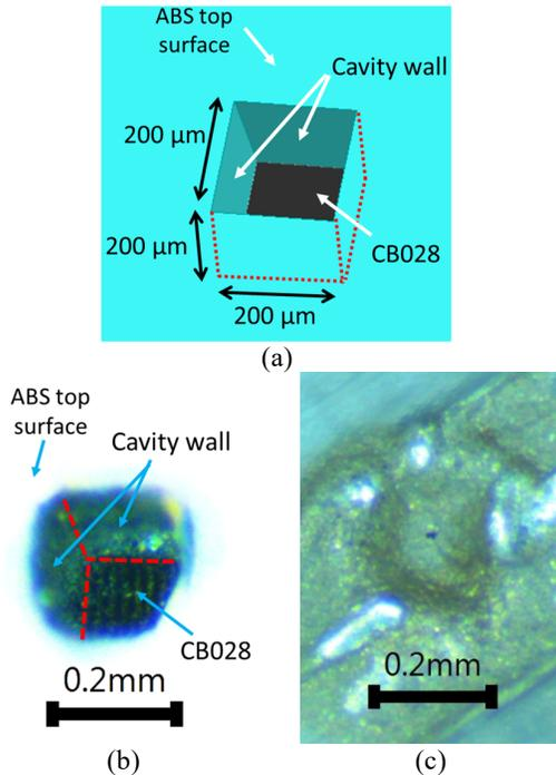
Figure 5: (a) Diagram of the thru via. (b) Micrograph of the laser machined cavity (tilted top view). (c) Thru via filed with CB028.
