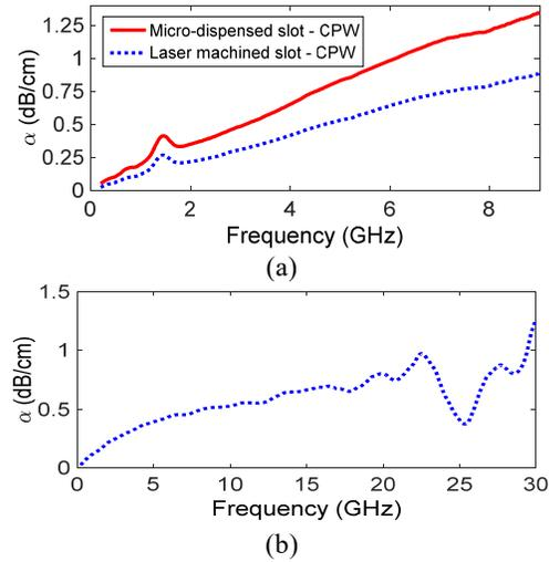
Figure 2. Measured loss of CPW: (a) micro-dispensed and laser machined 50  $\mu\text{m}$  wide slots. (b) Laser machined 20  $\mu\text{m}$  wide slots [6].
