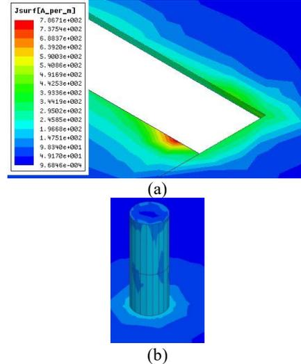
Figure 7: Simulated current densities on the resonator. (a) On the interconnect next to the post. (b) On the post.
