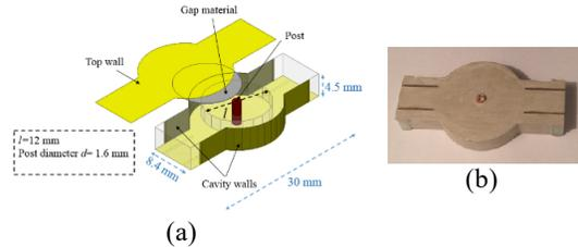
Figure 6: (a) Geometry of the cavity resonator. (b) Fabricated component [9].
