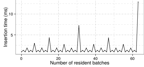
(a) Batch insertion time (ms) in GPU LSM with b = 2^{19} .
