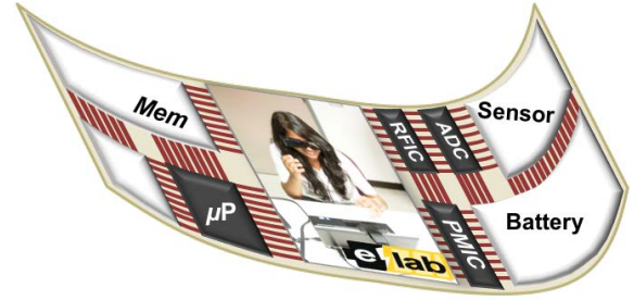
Figure 1: An illustration of flexible hybrid electronics system with flexible circuits, display, battery and rigid CMOS ICs.
