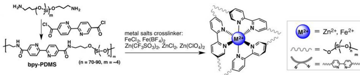
Figure 1. The synthetic route of metal salts cross-linked PDMS.
