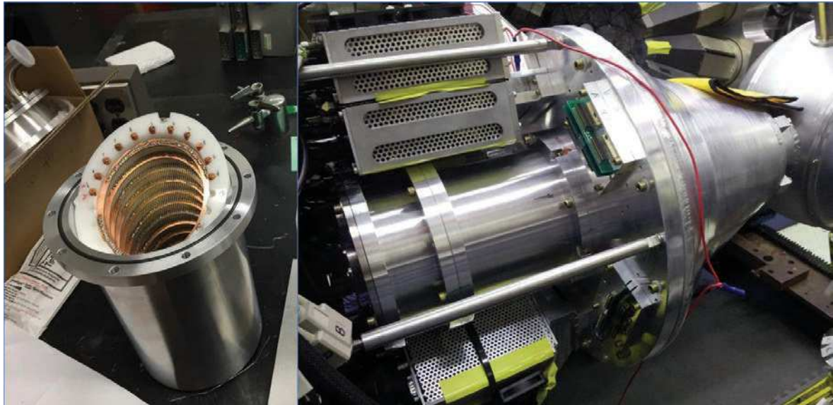
Fig. 2. Photo (left panel) of the front half of the compact tilted-grid fast ionization chamber, in which the grids can be seen, and (right panel) photo of the CTGFIC installed in the GODDESS setup, between the preamplifier boxes.
