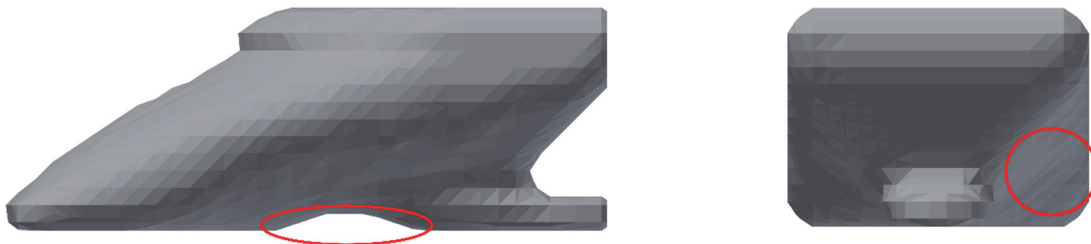
Fig. 28 Overhang areas with the inclination angle below 45 degree (marked out by the red circles)
