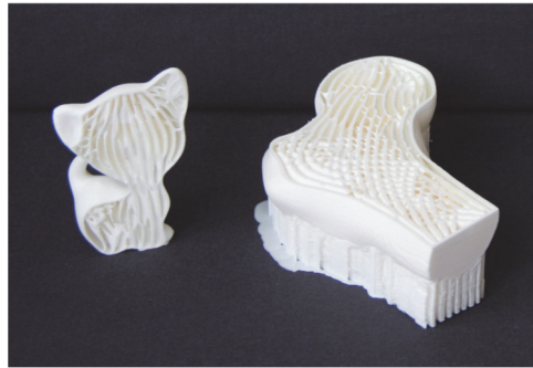
(a) High-resolution voxel-based porous infill (Wu et al. 2017)
