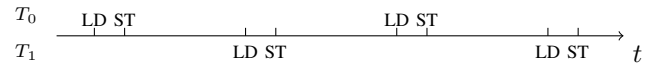
Fig. 3. The basic idea of the data race design. Monitoring the memory operations of the two threads on \mathcal{V} . LD: load; ST: store.
