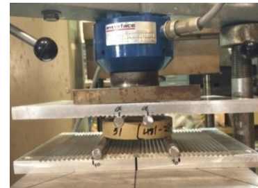
Figure A-2. View of Example Flat Ring Flexure Apparatus in Test Machine
