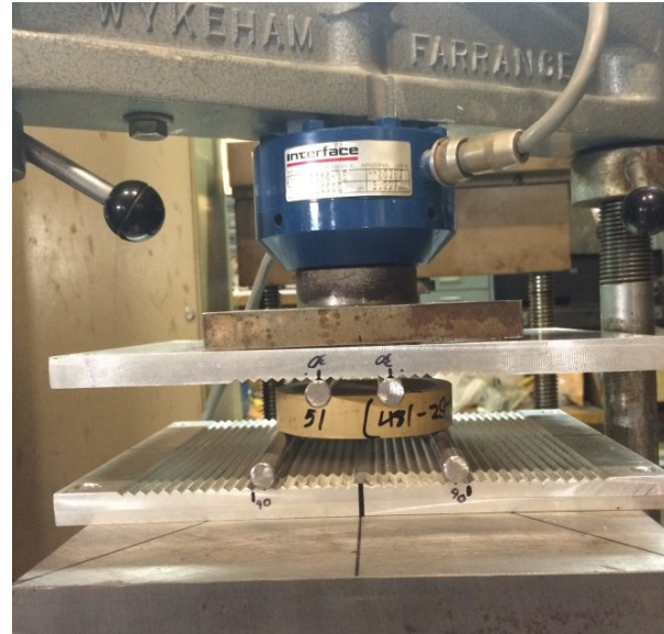
c) test being conducted in universal test machine (shown 100 mm diameter specimen tested over 80 mm span with 25 mm shear span)
