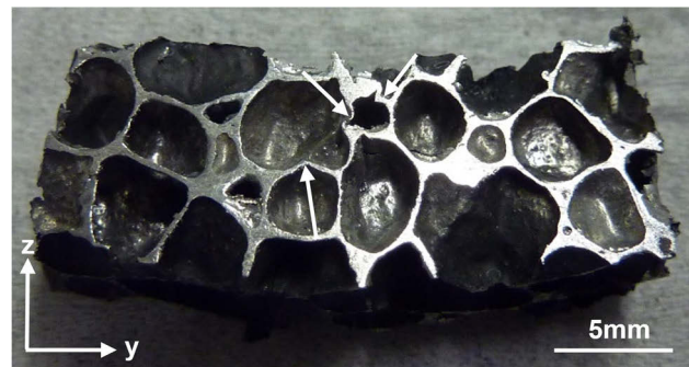
Fig. 5 Cross section of a foam specimen after five laser scans at 180 W and 10 mm/s. The laser was scanned into the page. The white arrows show where cell walls were bent during laser forming, indicating that the foam cannot withstand high compressive stresses.
