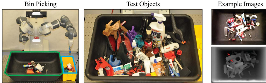
Figure 2: (Let) For each experiment, a subset of N validation objects are randomly dropped into a bin (green rim, center), at which point the YuMi iteratively plans grasps from point clouds and attempts to lift and transport the objects to a packing box (blue rim, right side). (Middle) A set of 50 test objects with various shapes, sizes, and material properties. A subset of 25 are rigid and opaque, and 25 others have transparency (e.g. goggles), moving parts (e.g. can opener), or deformable material (e.g. cloth). (Right) Example color and depth images from the physical setup with example grasp planned with the Dex-Net 2.1 \epsilon = 0.9 policy.
