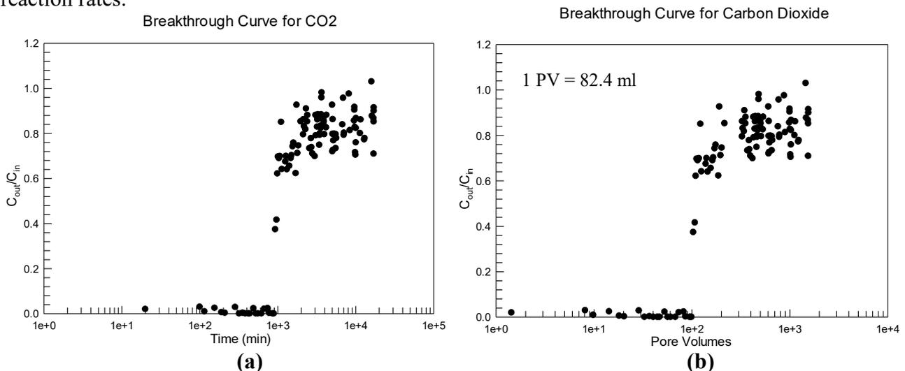
**Figure 4: Breakthrough Curve of Carbon Dioxide in Small Column Experiment with respect to (a) Time and (b) Pore Volumes**
