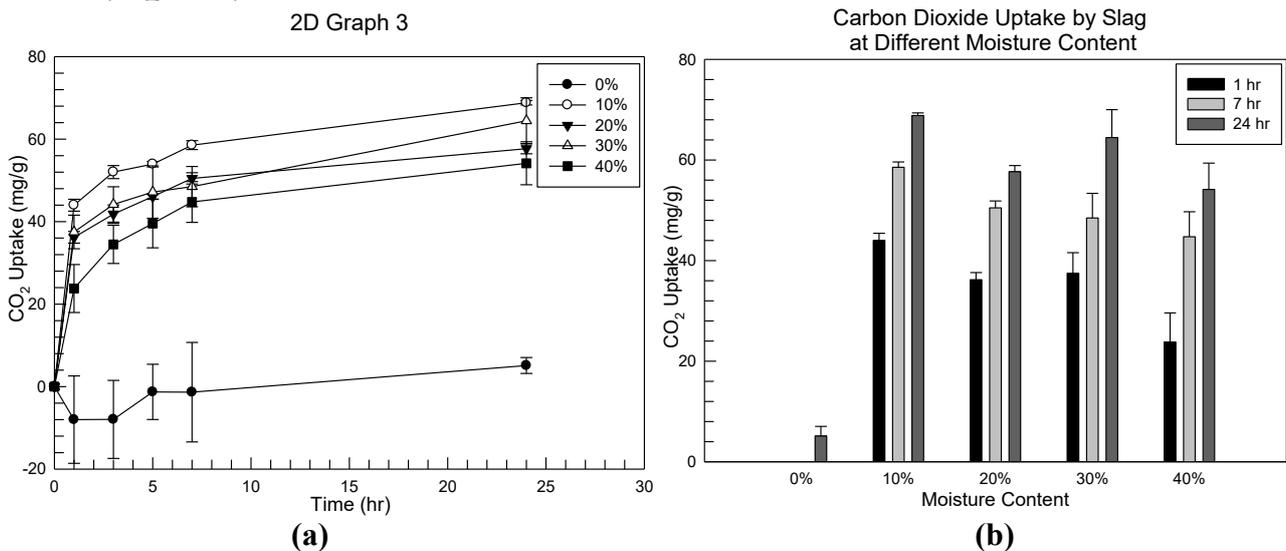
**Figure 3: Carbon Dioxide uptake by BOF Slag for Different Initial Moisture Contents**
