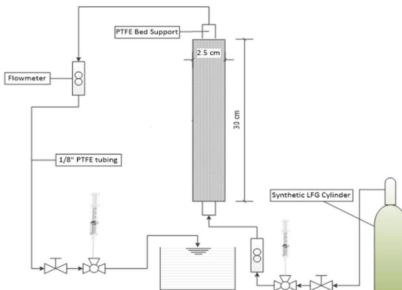
**Figure 2: Schematic of Column Experimental Test Setup**
