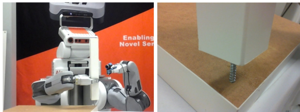
Fig. 1. The PR2 using a hand-held camera to view the table assembly task (left) and an example view of a successful attempt (right).
