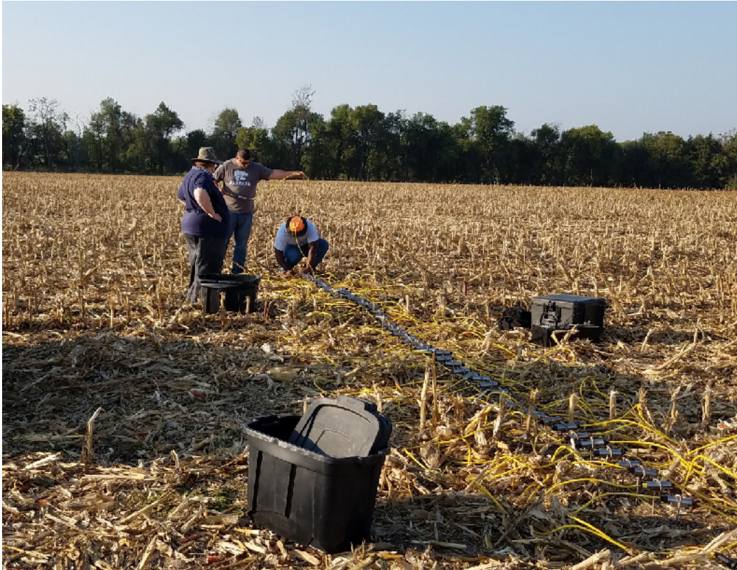
Figure 2. ERT survey experimental setup. Each stainless steel stake is 12 in. long and placed at half-foot intervals across the survey. The stainless steel electrodes are attached to the stainless steel stakes where an electrical current is transmitted through each electrode. The apparent resistivity measurements are recorded for each electrode and stored for later analysis to build the soil profile images presented in Figure 3.
