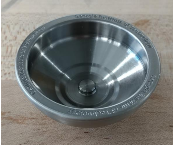
a. Product 18 after machining in first fixture
