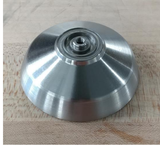
b. Product 18 after machining in second fixture
