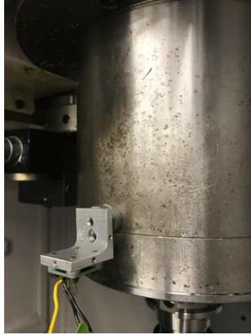
a. Accelerometer Mounted to Machine Tool Spindle
