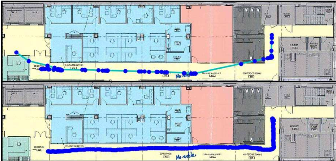
Fig. 7. Sample (estimated) trajectories captured by the apps during a navigation experiment. (Top: BLE; bottom: Hybrid). Users followed the instructions given by the app in walking forward (a certain number of meters/feet/steps), turning (left or right), and stopping; however, their actual trajectories differed from the estimated ones in that users did not bump into walls by using their cane/dog or our vibrotactile devices.
