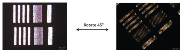
Fig. 6 Microscope images of uniaxial aligned stripe like structured LCE films between two crossed polarisers. On the left image LCE stripes and their director are at a 45° angle to crossed polarisers. On the right image the director of LCE stripes is parallel to one of the crossed polarisers. Dark and bright images proof that there is no loss of alignment after the patterning process (scale bar: 200 μm).
