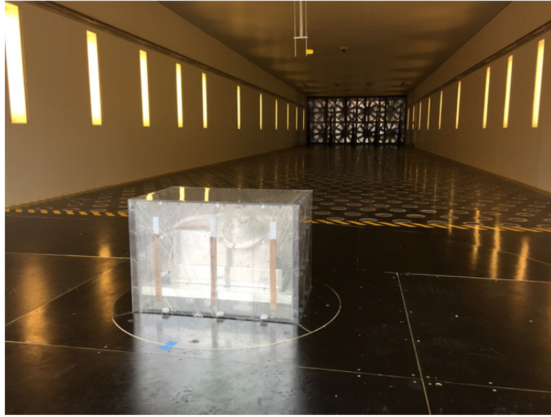
Figure 7. Boundary layer wind tunnel with model low-rise building, upwind view
