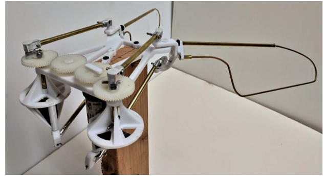
Fig. 11 Gear train and input cranks of the physical model of the flapping wing mechanism
