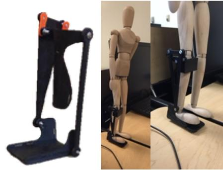
**FIGURE 17.** Reduced scale 3D printed model of the orthotic device.
