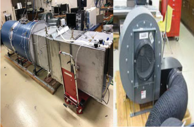
Figure 1: The air-flow bench and the Air Blower
