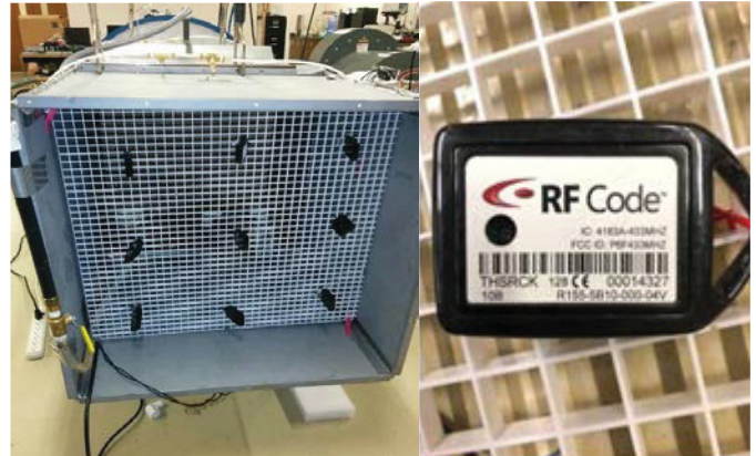
Figure 3: RF code R155 Humidity-temperature sensors
