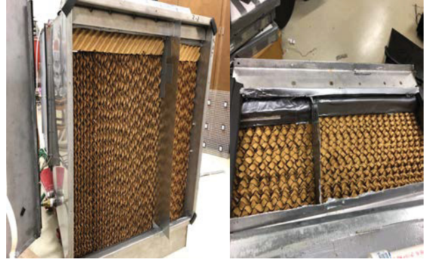
Figure 9: Side and top view of the DEC pad fitted inside the middle duct.
