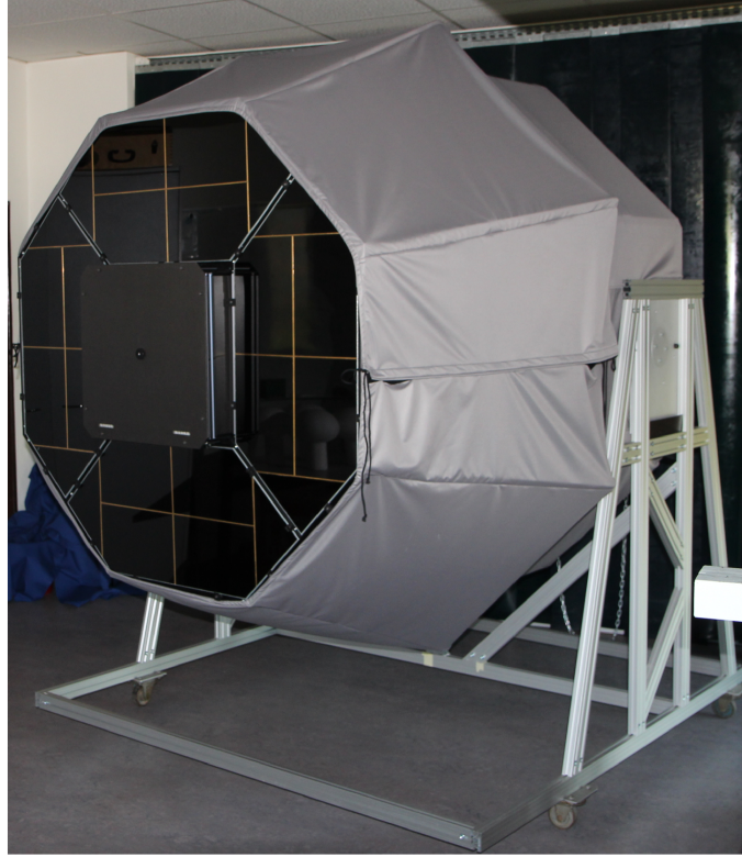
Figure 6. The complete mechanical structure. The mirror and the camera are protected from dust and aerosols by a shroud, which also acts as a shield for ambient light.
