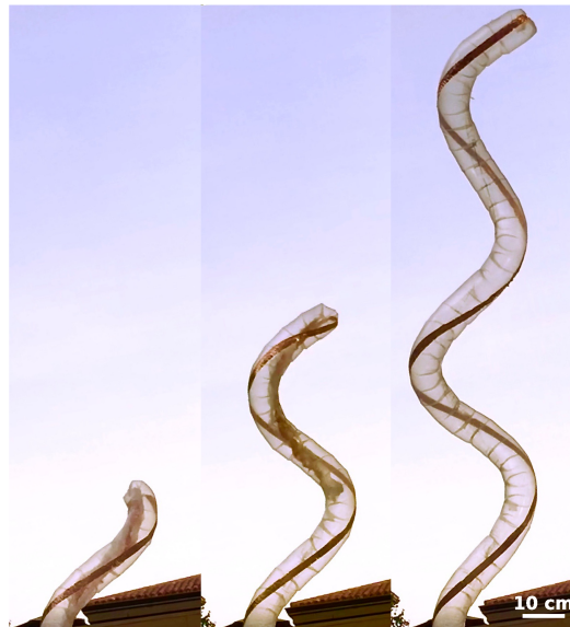
Fig. 1. A soft, inflated robot is grown into a helical antenna. Shape is mechanically pre-programmed by pinching the thin walled plastic tube along a line of actuation. Growth is achieved by feeding more material through the center to be everted at the tip, and the material is flexible but not stretchable.
