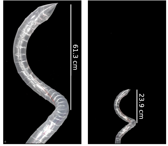
Fig. 6. Scaling up D by 2.5 times and holding \lambda and \theta constant leads to direct scaling of final shape parameters by 2.5 times as expected.
