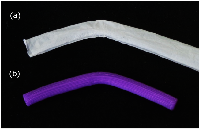
Fig. 3: (a) A pre-formed soft catheter. (b) The 3D-printed mold used to pre-form catheters.
