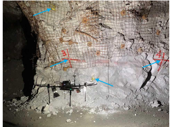
Fig. 4. Control points marked on the rib of the mine drift marked with spray paint (in red) and marked using a paintball gun (in yellow).
