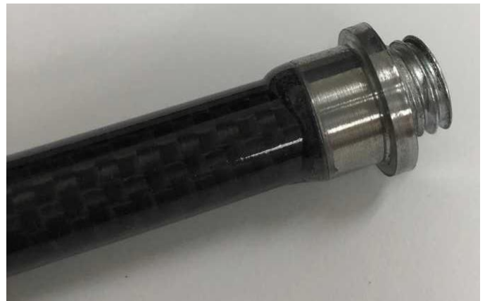
Fig. 3. Machined drain plug used to serve as UAV leg attachment piece.
