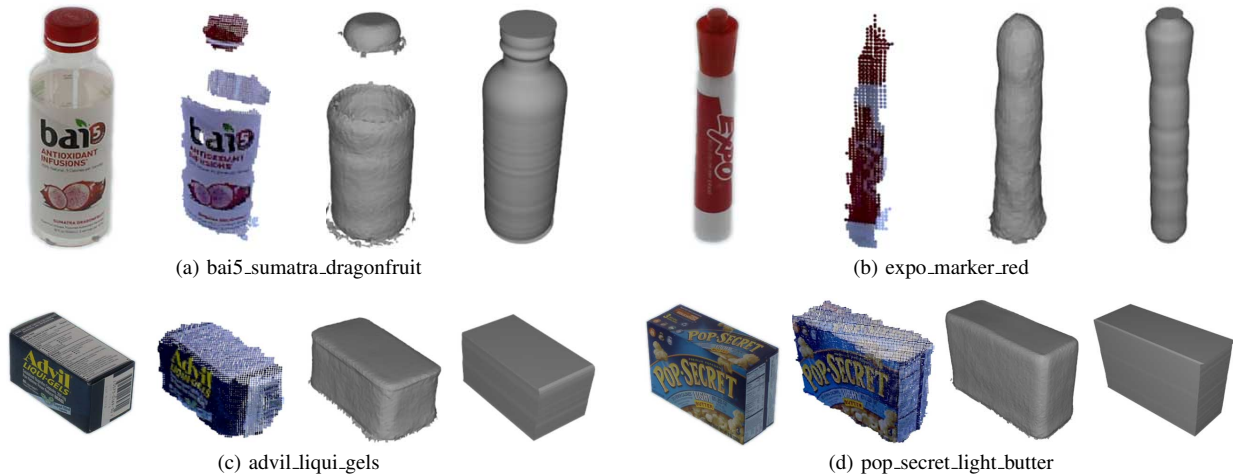
Fig. 5: Sample object extractions from the BigBIRD dataset. In each object group, the first column is the RGB image of the target object. The second column is the raw point cloud of the object. The third column is the ground truth mesh as provided by the BigBIRD dataset. The fourth column is the object modeled using our system. Refer to the accompanying video and the supplementary material for a full set of our extractions.
