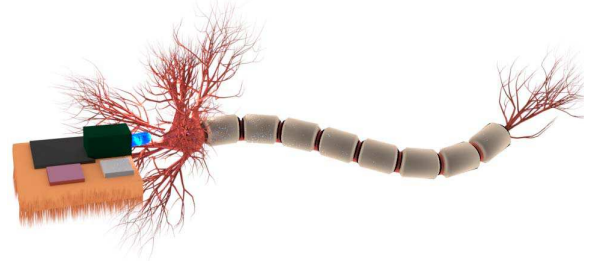
Fig. 4. Illustration of a WiOptND that interfaces to an engineered neuron that is sensitive to light at a specific wavelength.
