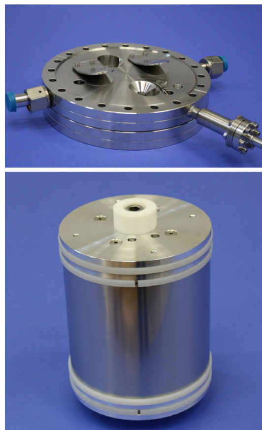
Fig. 8 Top: end flange containing gas-inlet and outlet, temperature sensor, feed-through and flapper valves. Bottom: magnetically-coupled, laser-welded piston with gaskets
