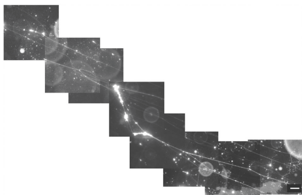
Fig. 2 Stitched epifluorescence images show inter-connected lipid tubules that are >1 mm in total length. Scale bar: 20 \mu\text{m} .
