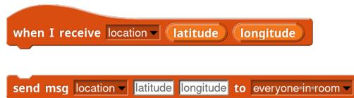
Figure 4: Sending and receiving messages with data in NetsBlox
