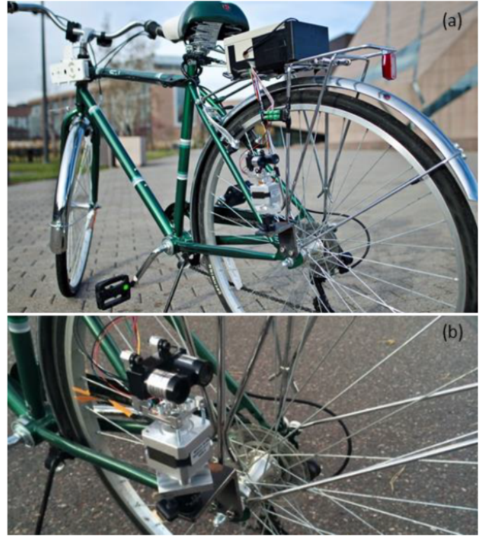
Fig. 2. Laser sensor system on bicycle. (a) Rear-facing sensor. (b) Zoomed in.
