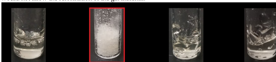
Figure 6. Photographs of solid PY-PSBTh broken xerogel (b) and reconstituted PY-PSBTh after standing at room temperature for 1 week (c), 2 weeks (d), and heating at 70 °C for 1 hour (a).
