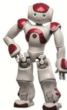
Fig. 1. Aldebaran's Nao robot is an autonomous, programmable humanoid robot.
