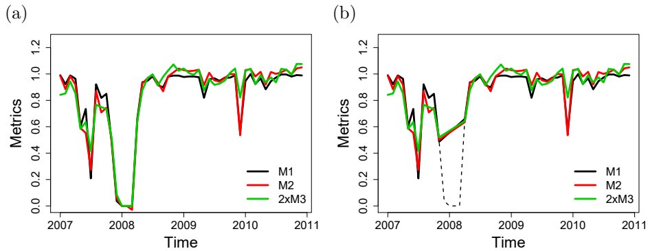
Figure 3: All three metrics plotted at monthly time resolution for WT1: (a) for the full period; (b) after eliminating the periods in which the turbine does not operate for most of the time (dashed line).
