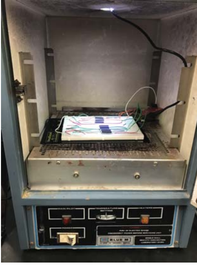
Fig. 10. Experimental setup to measure the reliability of the proposed solar cell based PUF against temperature variations
