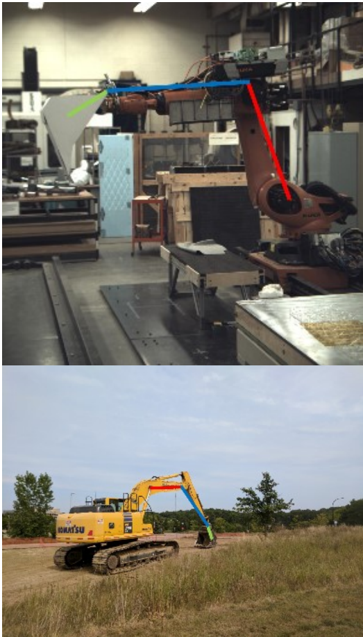
Figure 8. The result of the excavator pose estimation. On the top is the simulated excavator and on the bottom is the real excavator.
