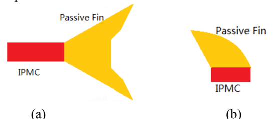
Figure 4. (a) Design of caudal fin; (b) design of pectoral fin.
