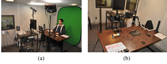
Figure 1: Data collection setting with the equipments used in the recordings of the CRSS-4ENGLISH-14 corpus [22].
