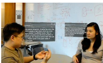
Figure 1a. Prototype 1: AR Windows displays captions in a HoloLens web browser window. Caption windows can be placed close to speakers or visual materials, such as lecture slides in 3D space.
