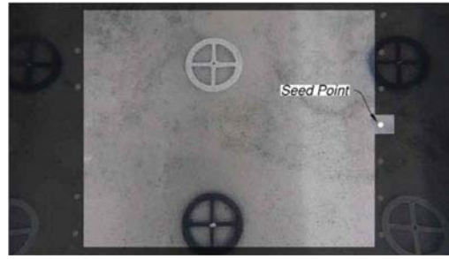
Figure 6. A typical view of a camera looking through the window. The gray area is the exclusion zone, the portions of the frame the GEOPIV software does not track displacements.
